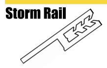
For replacing glass in windows. White PVC in 12' lengths.
